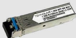
TGD-SFP Data Connections up to 1.25 Gbs Hot pluggable Duplex LC connector Up to 20 km at 9/125µm SMF Single +3.3V Power Supply Low power dissipation <1W typically Power dissipation <1.5W Industrial/Extended/Commercial operating temperature range: -40°C to 85°C/-5°C to 85°C/-0°C to 70°C Version available ROHS compliant and Lead-free
